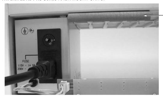
INSTALL SUPPLIED CONDUCTIVE FOAM GASKET (IFS P/N MMRFGSKT 375X500 or CHOMERICS P/N 82-122-74021-09600) CUT TO 4 INCH LENGTH AND PLACE ON TOP RAIL OF THE RACK WHERE THE UNIT IS TO BE INSTALLED.
