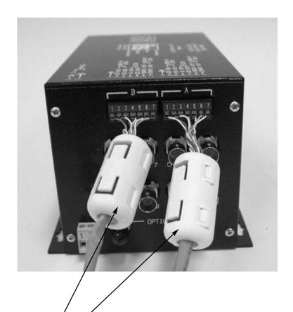
INSTALL SUPPLIED EMI FILTER CLAMPS (IFS P/N FL28A0640-0A0 or STEWARD P/N 28A0640-0A0) ON EACH DATA CABLE AS SHOWN.
