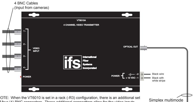
NOTE: When the VT6010 is set in a rack (-R3) configuration, there is an additional set of four (4) BNC connectors. These additional connecttors allow for the video inputs to be inserted from the front OR back of the unit BUT NOT BOTH.
