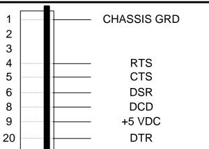
Blue jumper in position "A" of JP1 ties DSR permanently high. Blue jumper in position "B" of JP1 enables switch 2 to control DSR. Blue jumper in position "A" of JP2 ties DCD permanently high. Blue jumper in position "B" of JP2 enables switch 2 to control DCD. Blue jumper in position "A" of JP3 ties DTR permanently high. Blue jumper in position "B" of JP3 enables switch 2 to control DTR.
