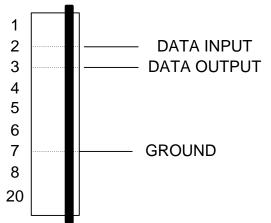
**NOTE:** DTE/DCE setting for RS-232 Data Output is controlled by switch SW1 ONLY.
