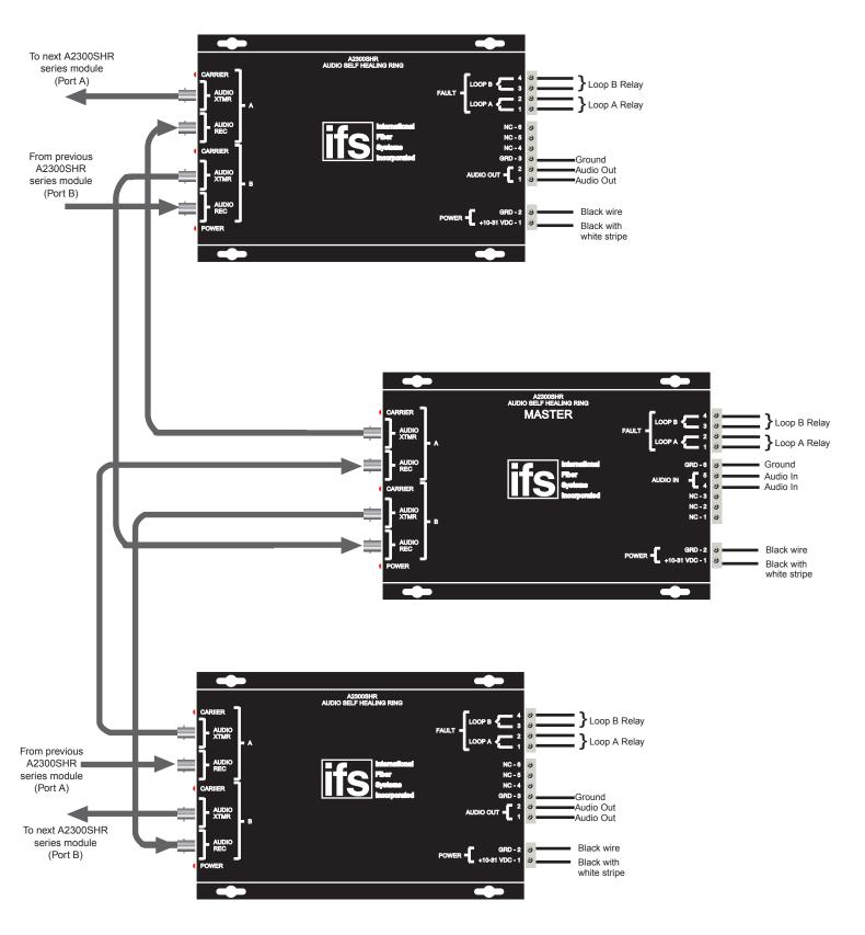
NOTE(S): The number of remote (repeater) modules is limited to 40.
