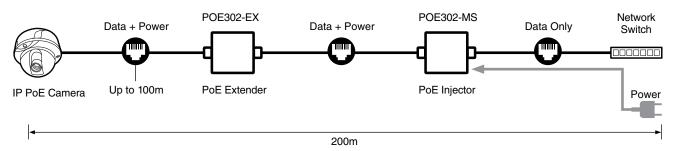
IFS Power over Ethernet (PoE) accessories provide quick and easy solutions for PoE challenges. A full range of IEEE 802.3-af or at compliant products allows for injecting, extending or splitting Power over Ethernet cable to provide extreme flexibility in handing PoE at the edge for powered devices, including IP-based Video, Access and Intercom, as well as VoIP and WAP applications.
