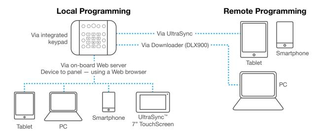
Multiple local and remote programming options provide customized configuration to best accommodate differing installations. UltraSync enables full remote system programming and device enrollment, reducing the need for truck rolls for scene and schedule creation, system adjustments or minor system add-ons.
