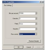
Power up the PB3 unit by plugging in the power supply. The following screen (or similar) will confirm that you are in HyperTerminal programming mode.
