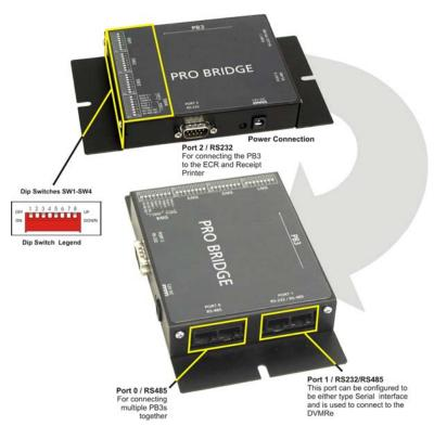
Figure 2-1. ProBridge Components.
