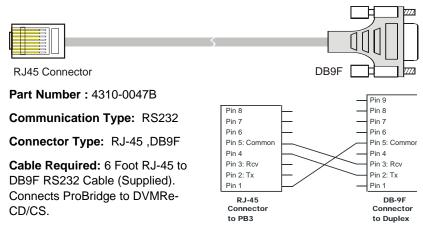
**NOTE**: This cable also used for Programming ProBridge via Windows
