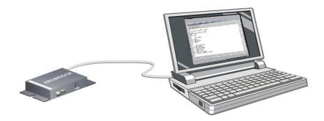
Figure 5-1. Laptop connected to PB3 running HyperTerminal.
