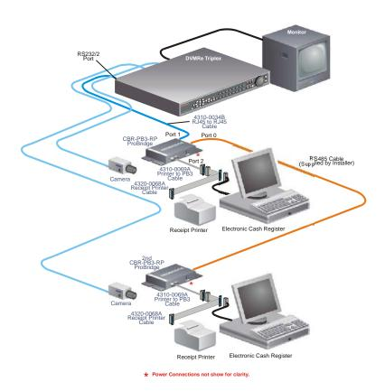
Figure 2-2. Typical System Layout.
