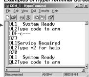
Status LED message - The Status LED message will be sent when the state of any of the displayed LED's change. The message will consist of "LDS", followed by 4 characters that represent the A(rmed), R(eady), F(ire), and P(ower) LED's. If the character position contains a hyphen (-), the corresponding LED is off. If the character is in lower case, the LED is on and if the character is in upper case, the LED is flashing.
