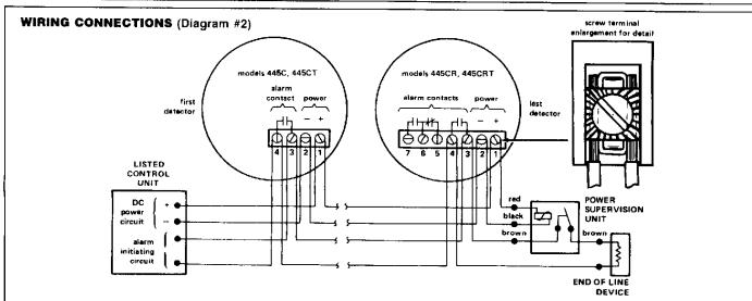
Emergency operation [Style D (Class A)]: Return initiating circuit wiring to appropriate control unit terminals and connect the end of fine devices per the control unit instructions.
