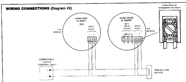
\*ESL 1500 Series Control Unit with BMB, ZEM. Styles B or D wiring. Maximum line resistance = 100 ohms. Compatibility Identifier is CO1.
