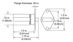
Note: In order to comply with UL installations, the contact should not be used on exterior doors that open outward.
