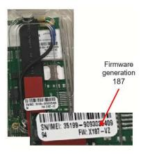
3. To find the exact modem firmware version, you can install the modem in a Simon panel and use the Interactive Services menu in System Programming to check the Module status. Below are screen shots showing how to find the module firmware version on the Simon XT and the Simon XTi-5i.
