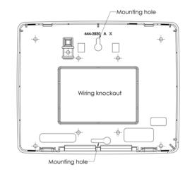
Secure the mounting screws (provided) to the locations on the wall marked in step 6. Do not tighten the screws. Leave enough clearance to mount the mounting plate.
