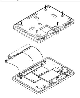
**Note:** If AC power is lost and battery pack is not present or depleted, the touch screen will not power up until AC power is restored (even if a new battery pack is installed).
