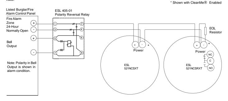
Note: The 405-03, 405-01, and 405-05 modules can be used with 4-wire 500N detectors, but only the 405-03 and the 405-01 can be used with 2-wire 500N detectors.
