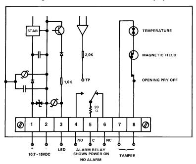
7.2 Connecting the DV1201 to a Four-wire Circuit Type Control in a UL Complete Mercantile Safe System
