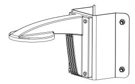
Mark the surface and drill four mounting holes. Install the corner mount adapter to the corner of a building using anchor B. Route the cables through the wall mount before bolting the corner adapter to the mounting surface.
