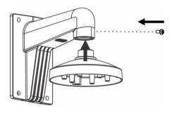
6. Place the adapter plate on the cup base wall mount. Prior to installing the adapter plate, make sure that when the camera is mounted to the adapter plate, it will be in the correct orientation. Using screw A, secure the adapter plate to the wall mount.
