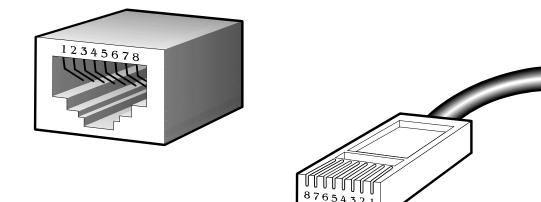
There are eight wires on a standard UTP/STP cable and each wire is color-coded. The following shows the pin allocation and the color of the straight cable and crossover cable connection:
