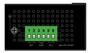
2. Tighten the wire-clamp screws to prevent the wires from loosening.
