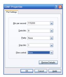
Log in to the console. After the terminal has been connected to the device, power on the managed switch. The terminal displays "running testing procedures".
