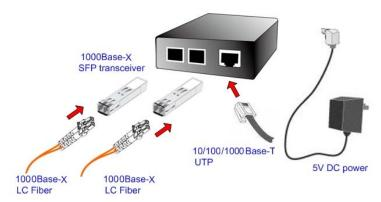
Figure 2-5-1: MCR300-1T-2S Gigabit Media Converter Stand Alone Installation
