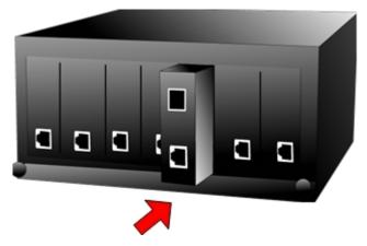
Figure 2-5-2: Insert a Gigabit Media Converter into an available slot
