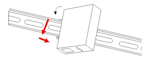
**Step 3:** Check the DIN-Rail is tightly on the track.
