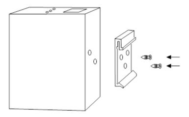
Step 2: Lightly press push the DIN-Rail into the track.
