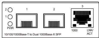
Figure 2-2-1: MCR300-1T-2S Front Panel
