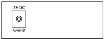
Figure 2-3-1: One DC jack for DC power input
