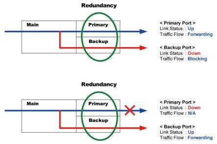
Figure 2-5: Redundancy Behavior Topology
