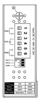
Figure 2-2: Industrial Gigabit Ethernet Switch Upper Panel
