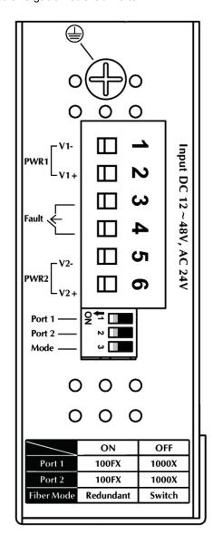
Figure 2-2: Industrial Gigabit Media Converter Upper Panel
