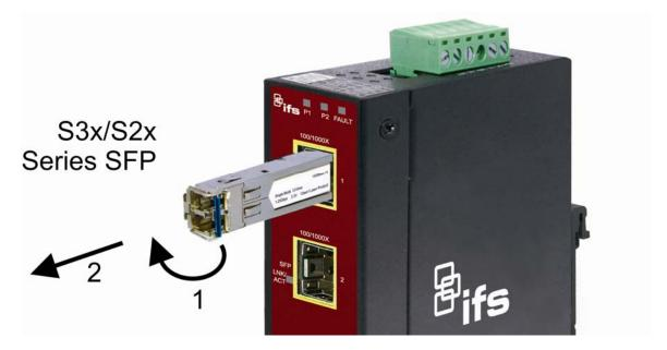
Figure 2-4: Pulling Out from the Transceiver
