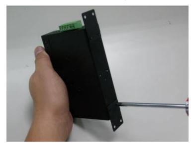
Step 3: Use the screws to screw the wall mount plate on the Industrial Gigabit Media Converter.
