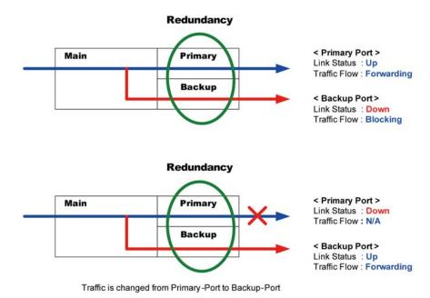
Figure 2-5: Redundancy Behavior Topology
