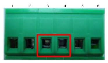
Insert the wires into the fault alarm contacts.
