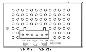
2. Tighten the wire-clamp screws for preventing the wires from loosening.
