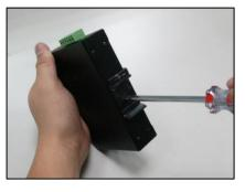
2. Place the bottom of DIN-rail lightly into the track.
