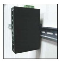
To remove the industrial fast Ethernet switch from the track, carefully pull out the bottom of the DIN-rail to remove it from the track.
