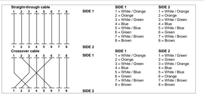
Ensure that the connected cables have the same pin assignment and color as described above.
