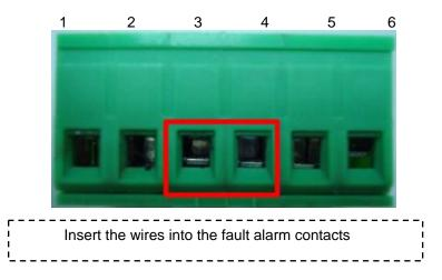
**Note:** The wire gauge for the terminal block should be in the range between 12 ~ 24 AWG.
