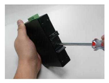
2. Place the wall mount plate on the rear panel of the MC251-4P/1S and the NS2051-4P/1T.
