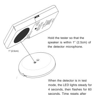
Figure 8. Using the Tester
