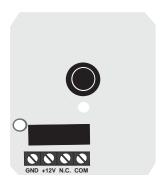
Figure 7. Wiring Terminals
