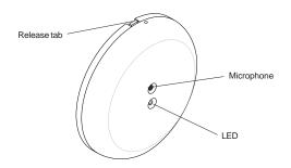
Figure 4. Housing Parts
