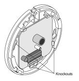
Figure 6. Detector Knockout Locations
