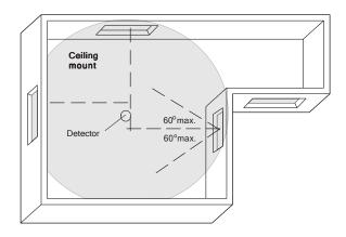
Figure 3. Multiple Window Coverage
