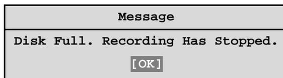
Unit will not record over previously recorded data. To continue recording, the data must be erased (or deleted) in the **Advanced**® **Disk Maintenance** menu.
