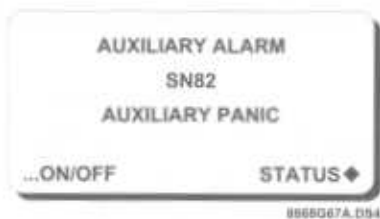
Figure 23. Auxiliary Panic Alarm Display
