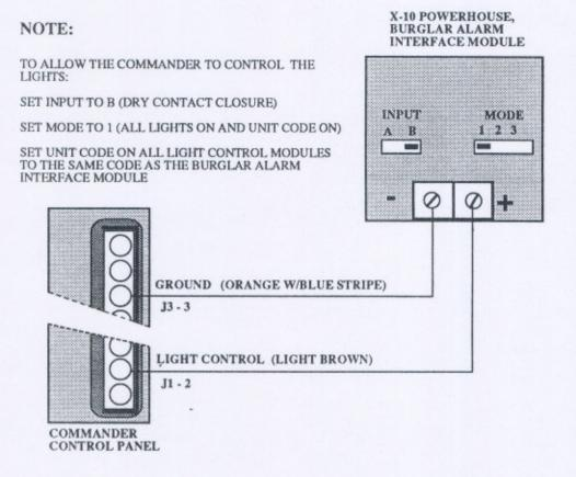
When wiring peripheral components to the Commander, you should always consider whether the device has a Normally Open or Normally Closed switch.
