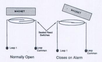
Of the components available from ITI for the Commander, only the Smoke, Heat detectors, and Panic buttons are Normally Open; all others are Normally Closed.
