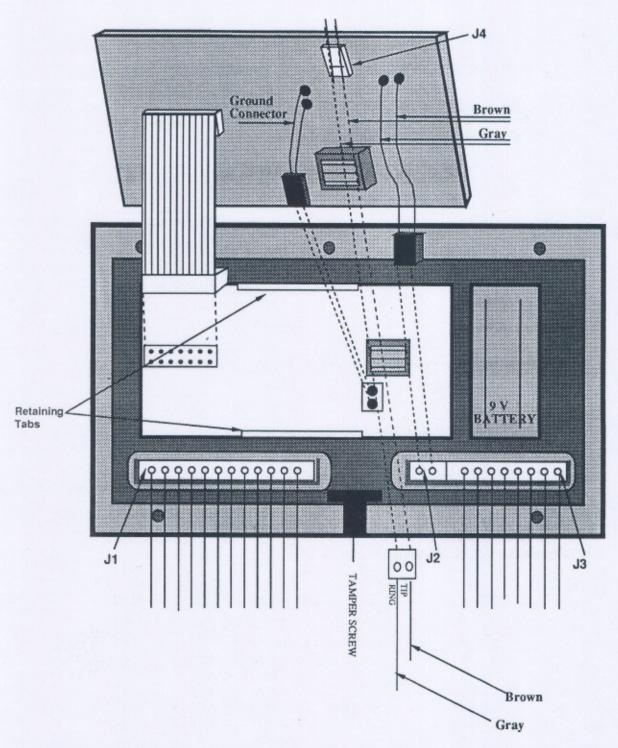
NOTE: When installing a Telephone Control Module, be sure all connections are good and the circuit board is snapped securely in place under the retaining tabs on the Control Panel.
