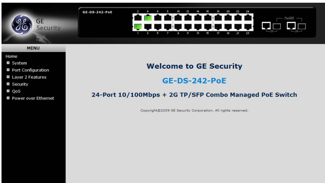
Figure 3-2: Web main screen of Managed Switch
