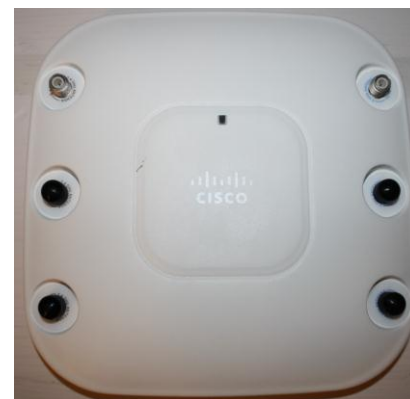
Figure 8. Black protective caps shown on four ports
