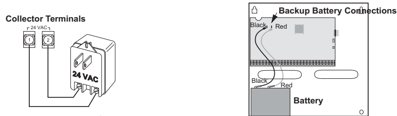
Figure 10: Connecting a Power Transformer and Backup Battery
