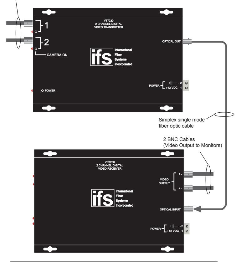
NOTE: WITHOUT PROPER FIBER CONNECTION, LED'S DO NOT INDICATE CORRECT OPERATIONAL STATUS OF THE UNIT.
