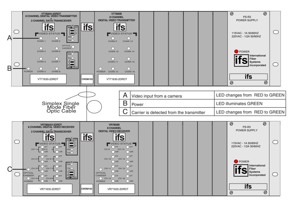
NOTE: WITHOUT PROPER FIBER CONNECTION, LED'S DO NOT INDICATE CORRECT OPERATIONAL STATUS OF THE UNIT.
