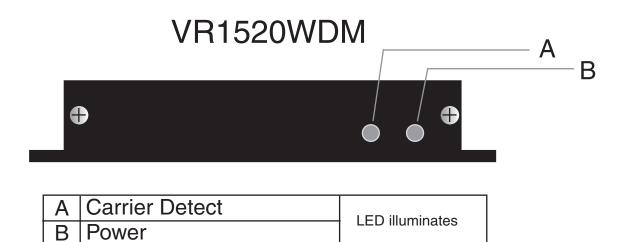
NOTE: WITHOUT PROPER FIBER CONNECTION, LED'S DO NOT INDICATE CORRECT OPERATIONAL STATUS OF THE UNIT.
