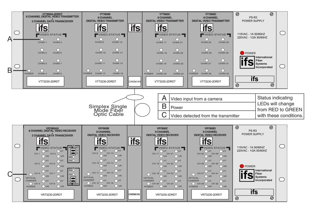
NOTE: WITHOUT PROPER FIBER CONNECTION, LED'S DO NOT INDICATE CORRECT OPERATIONAL STATUS OF THE UNIT.
