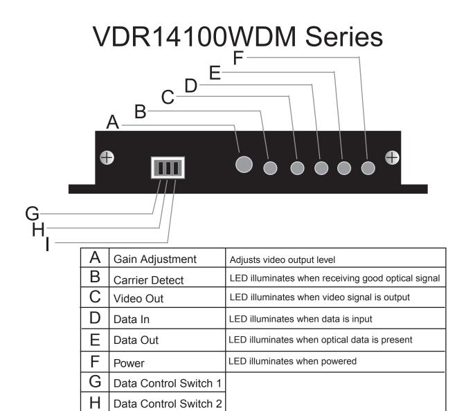
NOTE: WITHOUT PROPER FIBER CONNECTION, LED'S DO NOT INDICATE CORRECT OPERATIONAL STATUS OF THE UNIT.
