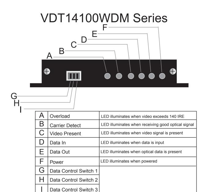
NOTE: WITHOUT PROPER FIBER CONNECTION, LED'S DO NOT INDICATE CORRECT OPERATIONAL STATUS OF THE UNIT.
