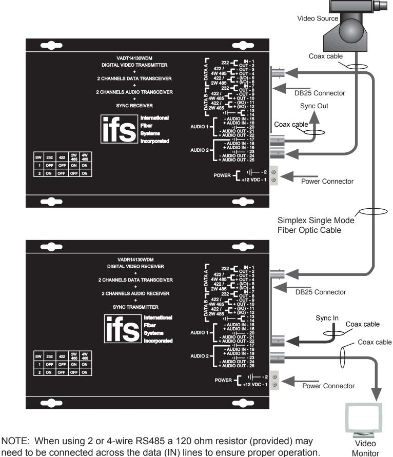
need to be connected across the data (IN) lines to ensure proper operation.
