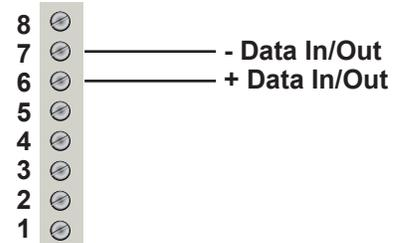
NOTE: A 120 ohm resistor (provided) may need to be connected across the data lines to ensure proper operation.
