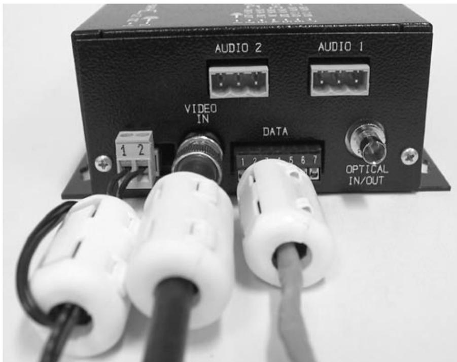
INSTALLATION INSTRUCTIONS FOR ADDITIONAL COMPONENTS REQUIRED TO MEET **EMISSION REQUIREMENTS** ON THE **VAADT14130WDM Series** STAND ALONE UNIT. (5 CLAMPS REQUIRED).
