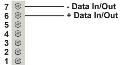
NOTE: A 120 ohm resistor (provided) may need to be connected across the data lines to ensure proper operation.
