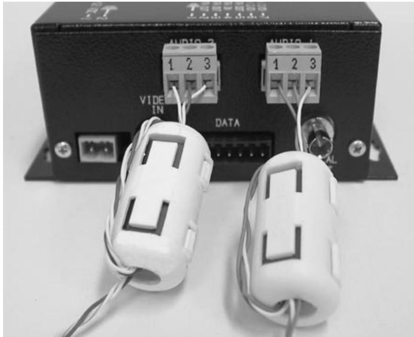
INSTALL SUPPLIED EMI FILTER CLAMPS (IFS P/N FL28A0640-0A0 or STEWARD P/N 28A0640-0A0 ON EACH CABLE AS SHOWN.
