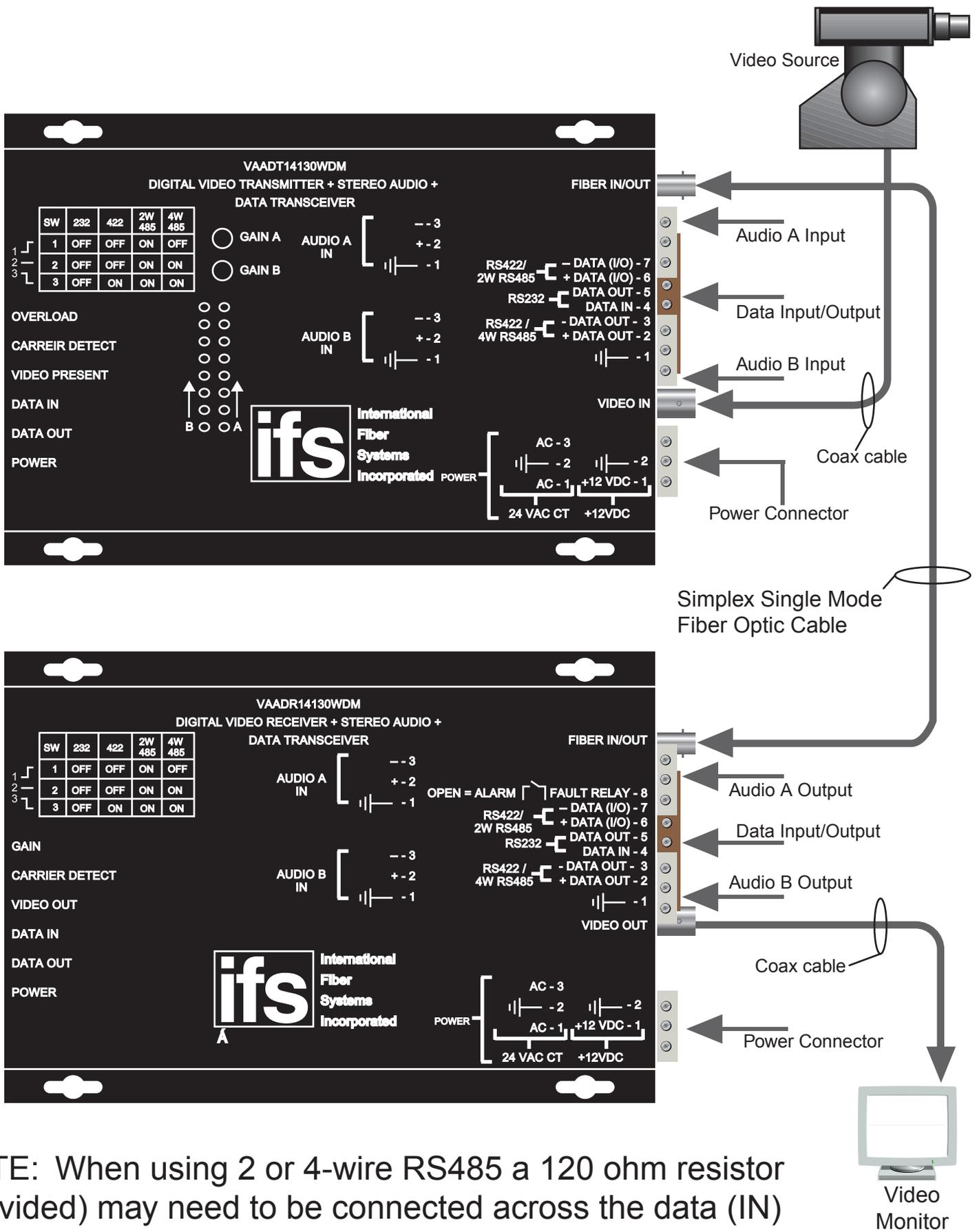
NOTE: When using 2 or 4-wire RS485 a 120 ohm resistor (provided) may need to be connected across the data (IN) lines to ensure proper operation.
