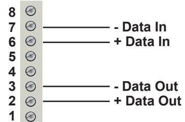
NOTE: A 120 ohm resistor (provided) may need to be connected across the data (IN) lines to ensure proper operation.
