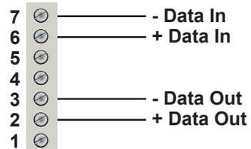
NOTE: A 120 ohm resistor (provided) may need to be connected across the data (IN) lines to ensure proper operation.
