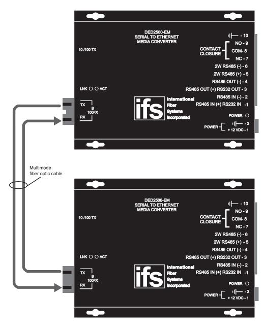
NOTE: When using 2 or 4-wire RS485 a 120 ohm resistor (provided) may need to be connected across the data (IN) lines to ensure proper operation.
