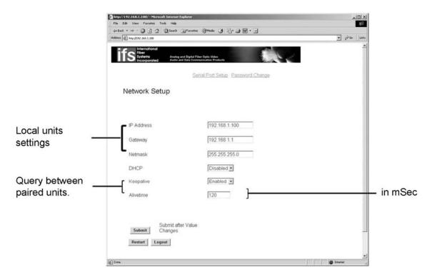
To set up the serial port, select the Serial Port Setup at the top of the Network Setup window. **Note:** The serial port must be configured prior to physically wiring the data port.
