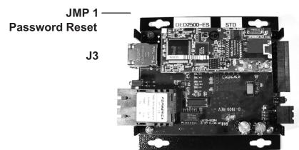
**To reset to factory defaults**, with no power applied to the unit, short the pins on JMP 1, then power the unit up for approx. 5 seconds. Power down and remove the short on JMP 1.
