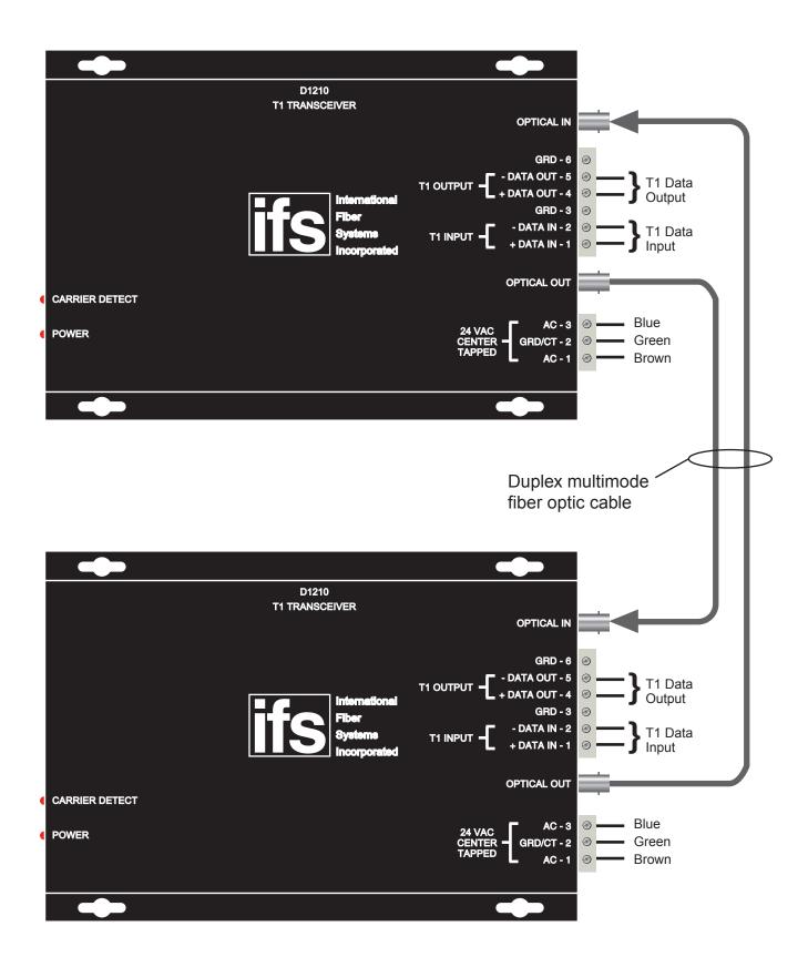
NOTE: In the event that the D1200 series modules are not operating correctly, the resistor that was included ma y need to be placed across the Data output lines (- Data Out to + Data Out).
