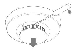
Figure 11: Removing the optical chamber
