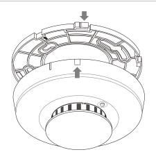
Figure 4: Detector installation
