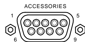
DB-9 Connector on Rear Panel
