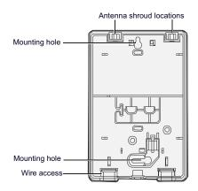
B. Drill holes and insert the appropriate anchors (included).
