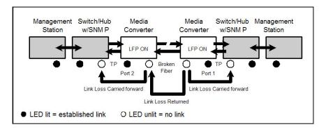
**Note:** LFP function is turned-off by default. This feature can also be enabled or disabled via the side DIP-switch. If the installer is familiar with the network installation and diagnostics (i.e. checking which end is broken in a connection), switch can be set to ON position and converter should be reset for changes to take effect. Otherwise, it's recommended to keep the DIP switch in its default position.
