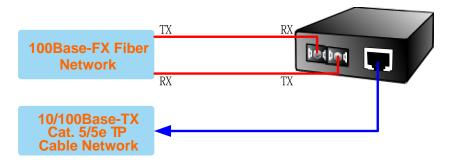
**Note:** RJ-45/STP, UTP Cat 5, straight /crossover cable is accepted.
