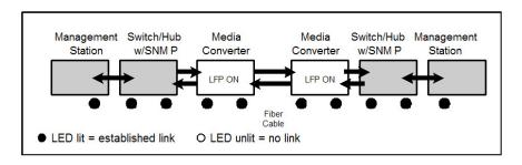
If one of the optical conductors is bad (as shown in the diagram box below), the fiber converter with LLR function will return a no-link condition to its link partner. With LLCF function also enabled, the no-link condition is carried forward to the switch/hub where a trap is generated to the management station.
