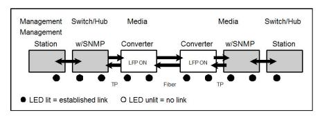
In case of a connectivity issue, the MC201-1T/1FS media converter LLCF sends the notification to the switch/hub that generates a trap to the management station.
