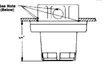
NOTE: Postive air pressure from wire openings, conduit, mounting boxes irregular mounting surfaces, or plenums causing air movement through and away from the detector may prevent proper operation. Seal all such openings causing unwanted air flow using UL Listed expanding foam or Duxseal.
