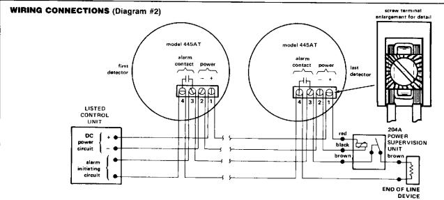
Emergency operation [Style D (Class A)]: Return initiating circuit wiring to appropriate control unit terminals and connect the end of line devices per the control unit instructions.
