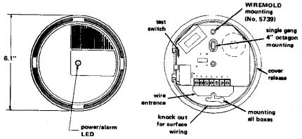
NOTE: Positive air pressure from wire openinge, conduit, mounting boxes, irregular mounting surfaces, or plenums causing air movement through and away from the detector may prevent proper operation. Seal all such openings causing unwanted air flow using UL Listed expanding foam or Duxseal.
