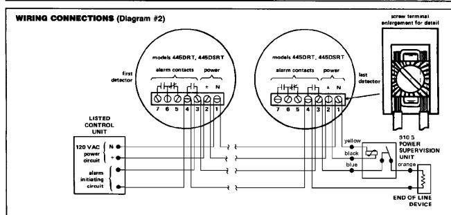
Emergency operation [Style D (Class A)]: Return initiating circuit wiring to appropriate control unit terminals and connect the end of line devices per the control unit instructions.
