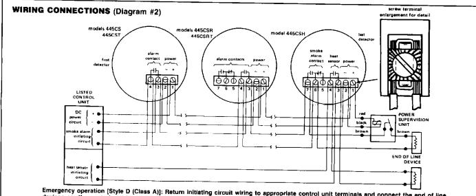
Emergency operation [Style D (Class A)]: Return initiating circuit wiring to appropriate control unit terminals and connect the end of line devices per the control unit instructions.
