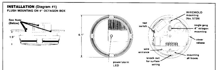
NOTE: Positive air pressure from wire openings, conduit, mounting boxes, irregular mounting surfaces, or plenums causing air movement through and away from the detector may prevent proper operation. Seal all such openings causing unwanted air flow using UL Listed Expanding Foam or Duxseal.
