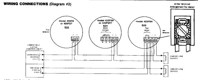
\*ESL 1500 Series Control Unit with BMB, ZEM. Styles B or D wiring. Maximum line resistance = 50 ohms. Compatibility Identifier is C01A.
